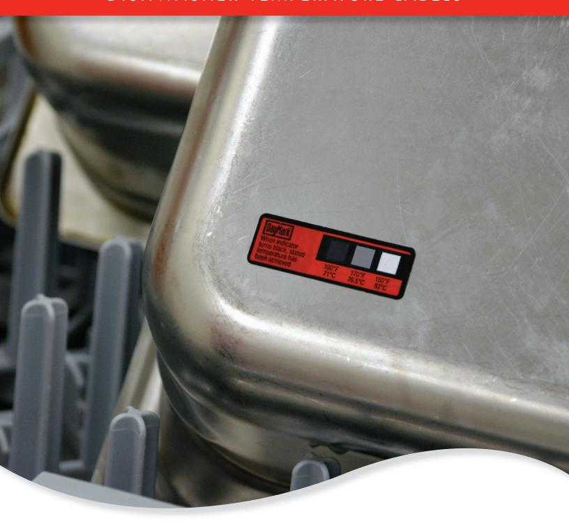
DayMark's Thermostrip® labels clearly and efficiently confirm that sanitation temperatures have been achieved in a commercial dishwasher, satisfying Section 4.7 of the Food Code—which calls for measuring sanitized food contact surfaces and utensils by an irreversible registering temperature indicator.
